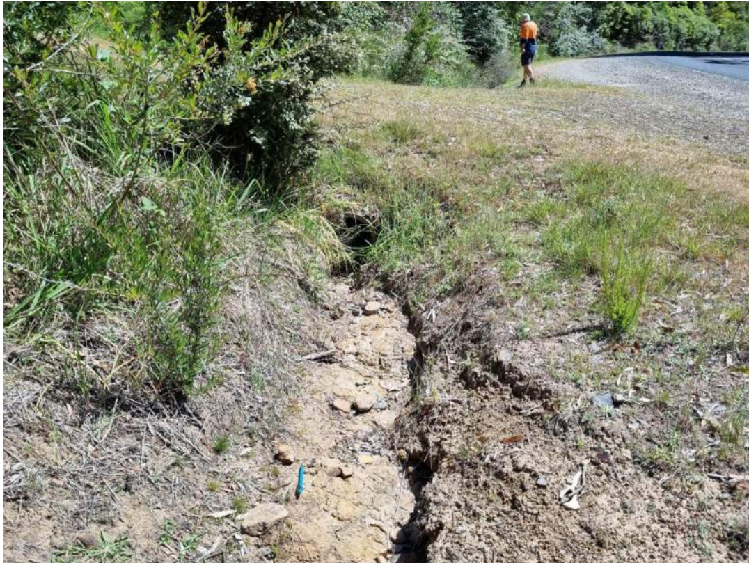
Photo 1: Dolerite bedrock exposed in drain on Deviot Road, opposite site driveway entrance, looking north-northwest.
