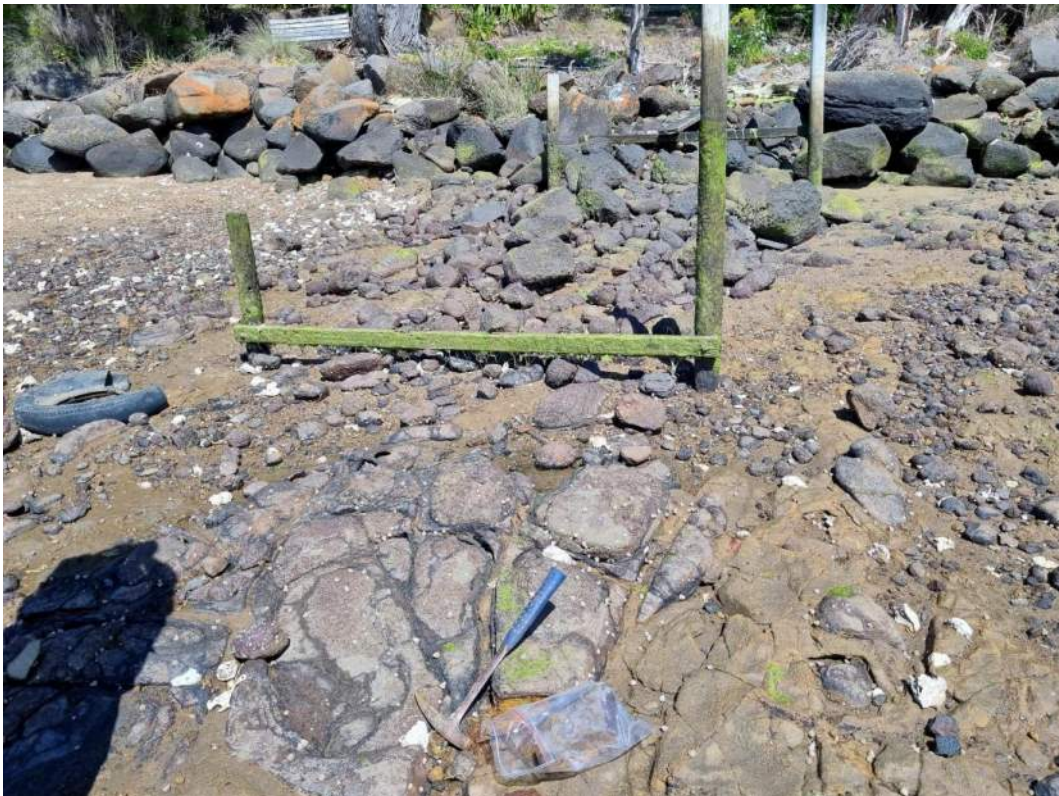
Photo 10: Moderately to Highly Weathered dolerite bedrock (Rock Sample location, RS3), and remnants of timber jetty/pier on foreshore to the east of the site, looking southwest. Note spherical or “onion-skin” weathering in the dolerite.
