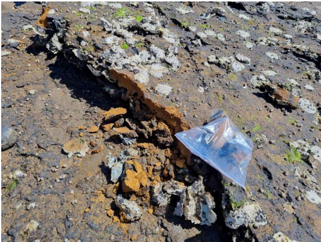
Photo 12: Highly Weathered sandstone bedrock (Rock Sample location, RS4) outcropping on foreshore to the east of the site.
