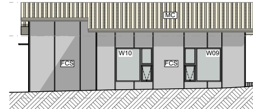
6.NE UNIT 6 North-East Elevation 1:100
