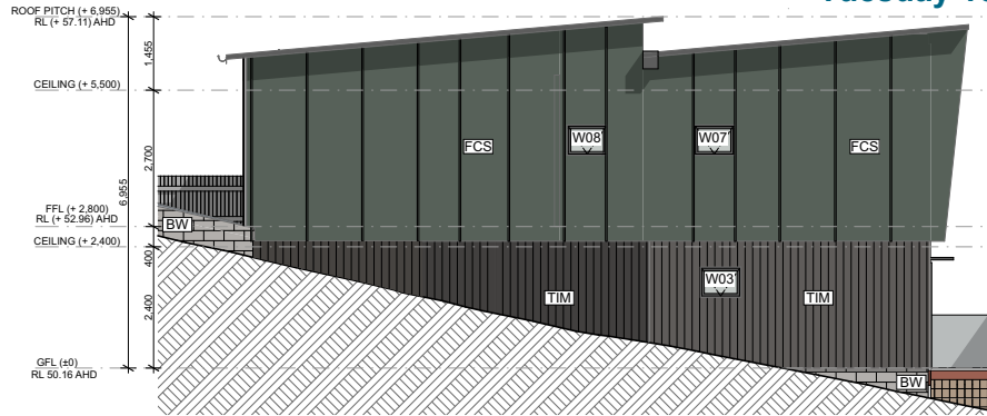
5.SE UNIT 5 South-East Elevation 1:100
