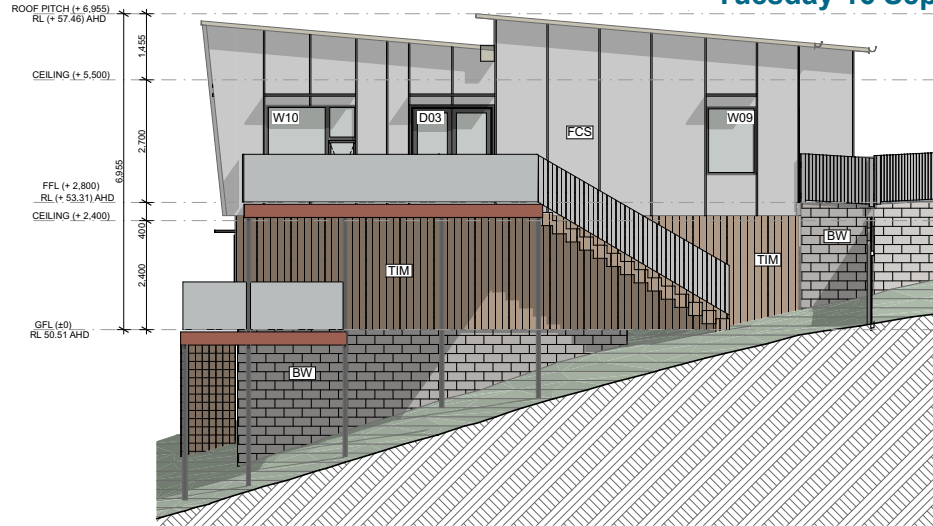
4.NW UNIT 04 North-West Elevation 1:100
