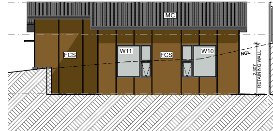
FCS HARDIE FLEX SHEET WITH BATTENS PAINTED FINISH TERRAIN
