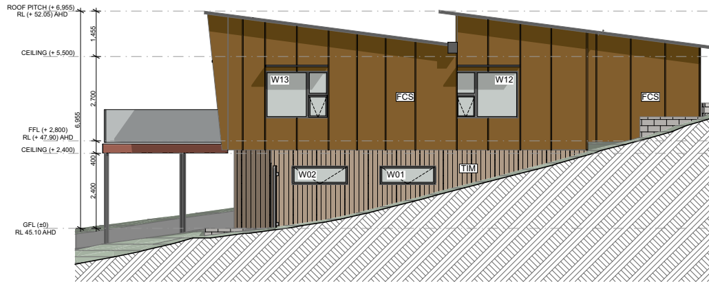
3.NW UNIT 03 North-West Elevation 1:100
