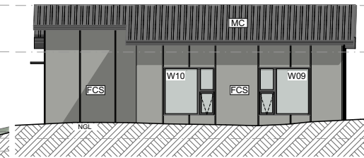
1.SW UNIT 01 South-West Elevation 1:100
