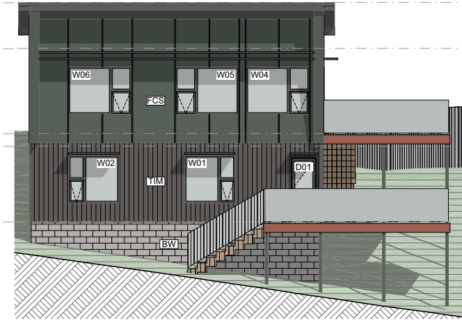
5.NE UNIT 5 North-East Elevation 1:100
