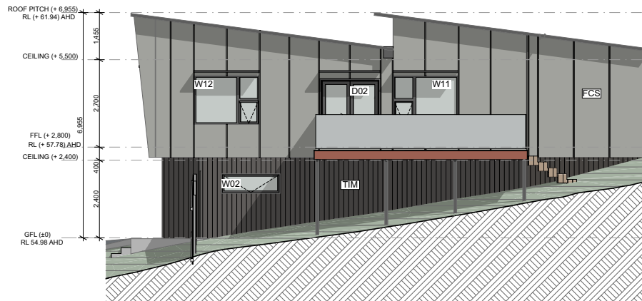
10.NW UNIT 10 North-West Elevation 1:100
