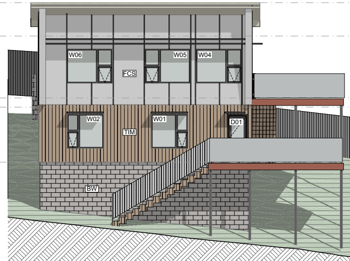
4.NE UNIT 04 North-East Elevation 1:100
