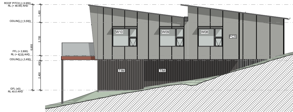
1.NW UNIT 01 North-West Elevation 1:100
