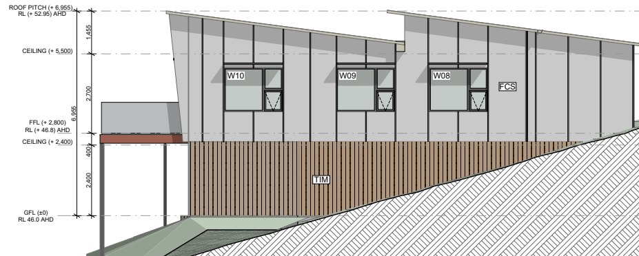
6.NW UNIT 6 North-West Elevation 1:100
