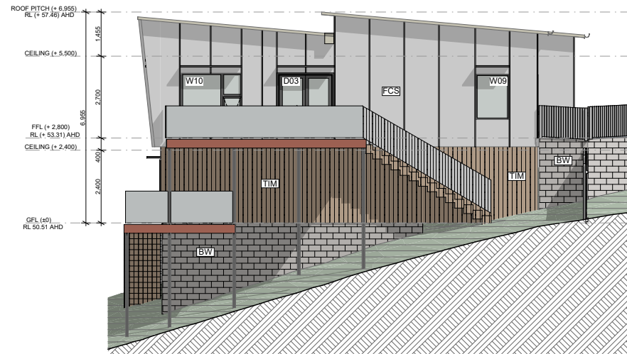
4.NW UNIT 04 North-West Elevation 1:100
