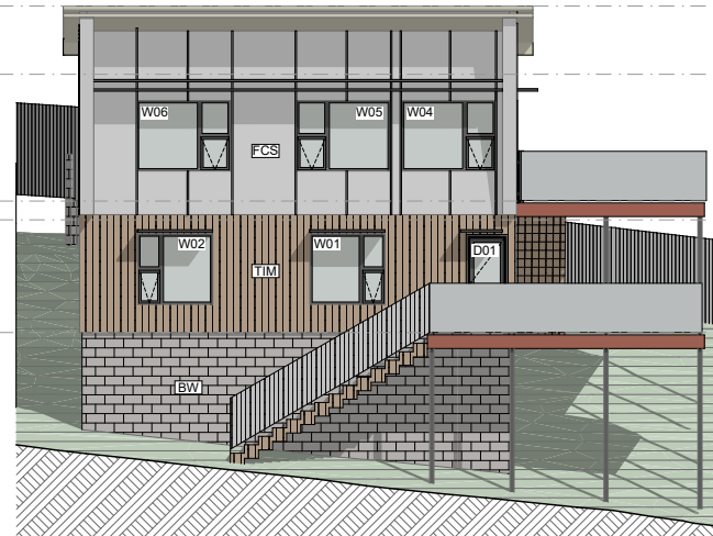
4.NE UNIT 04 North-East Elevation 1:100
