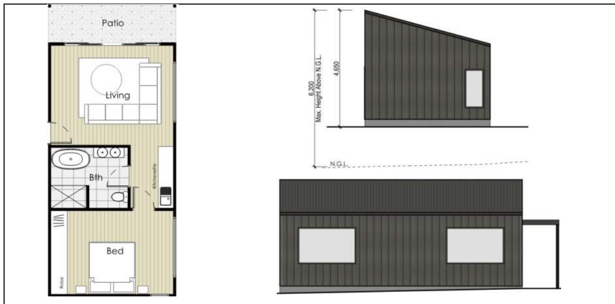
Figure 5 – Floor Plan (left), Elevations - North/East (right) – Building 1A. Source: Coactive Building Design
