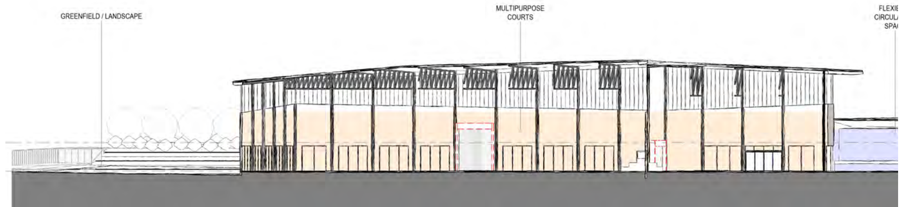
SITE SECTION (NOT TO SCALE) - SHOWING CONNECTIONS BETWEEN EACH FACILITIES AND RELATIONSHIP BETWEEN NATURAL GROUND LEVEL, EXISTING FOOTBALL GROUND LEVEL AND PROPOSED LEVELS
