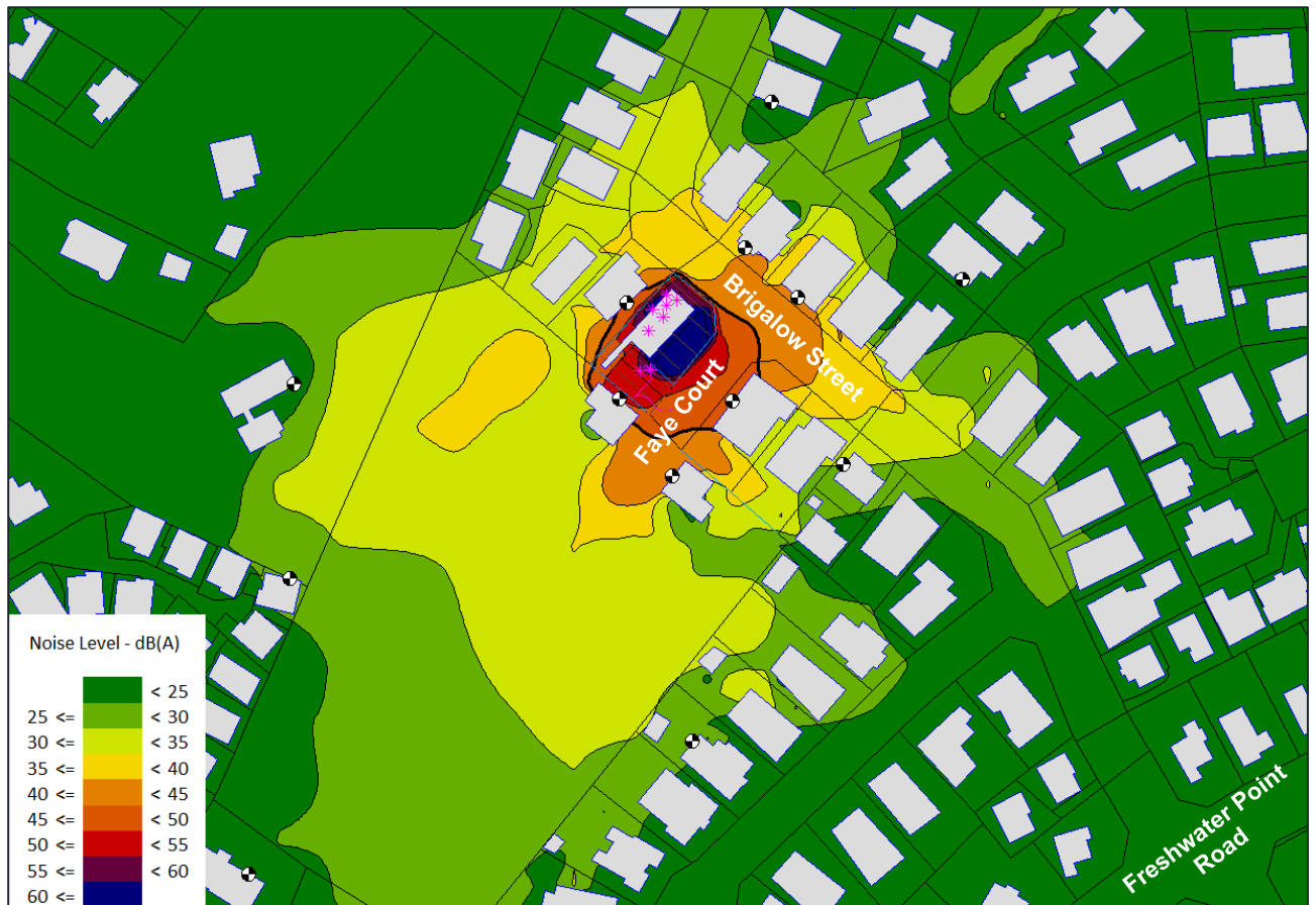
Figure 4: SoundPLAN noise grid map, for all sources operating, 45 dB(A) contour line shown in bold.
