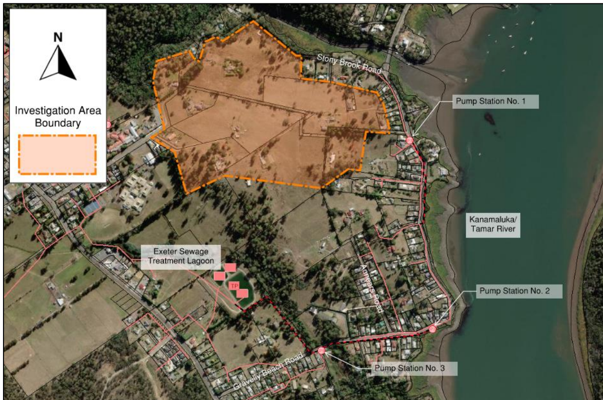
Figure 2 - aerial map illustrating the location of the three pressurised sewer tracts and associated sewer pump stations that service parts of the Blackwall residential area.
