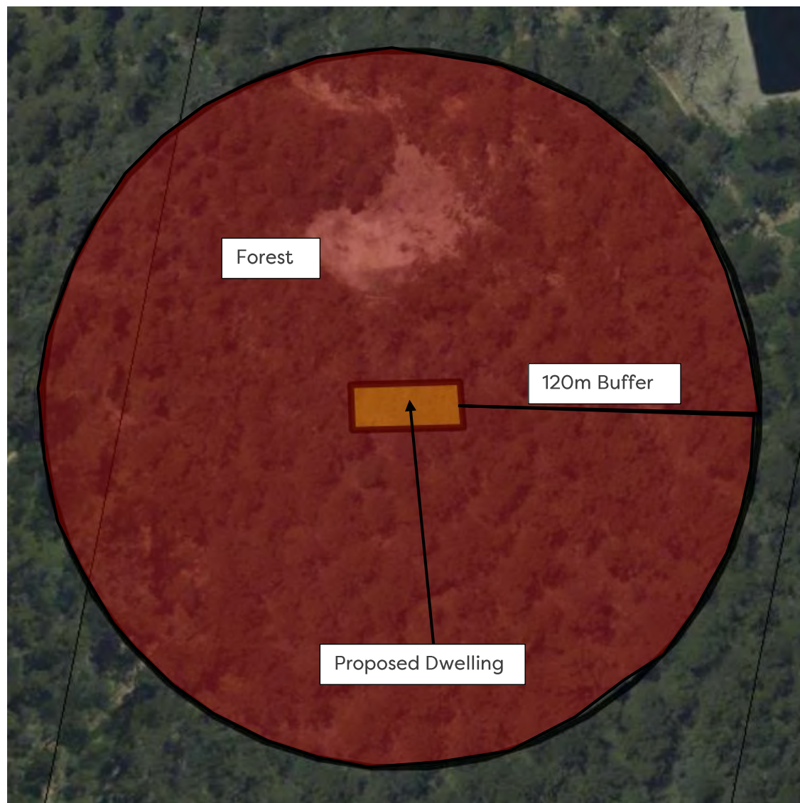
Figure 2 – Class building site with 120m vegetation.
