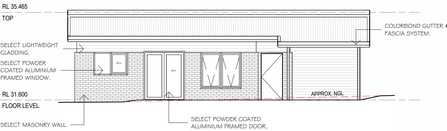
NORTH ELEVATION SCALE 1 : 100
